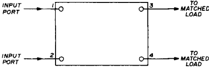
fig. 1. Block diagram of hybrid coupler. This device divides power between two matched loads.
